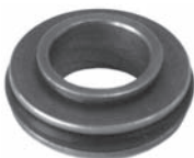
250649 Std pkg 5 Servicing FS6 O.D. 29.5 mm, I.D. 16.3 mm, Th. 10.7 mm Seal plate w/ extractor lip and O-ring
