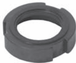
251298 Std pkg 10 Servicing DKV-14B O.D. 30 mm, I.D. 18.5 mm, Th. 7.75 mm Seal for head w/ O-ring (Neoprene)
