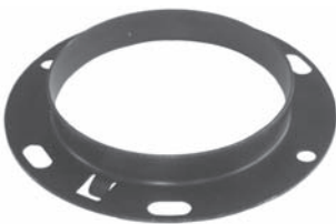
252248 Std pkg 10 Servicing 6SEU12C O.D. 98 mm, I.D. 66.6 mm, Th. 12.1 mm Washer
