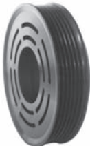
252388 Servicing SD6V12 O.D. 125 mm, bore 51 mm, W. 37.5 mm, 6 grooves
