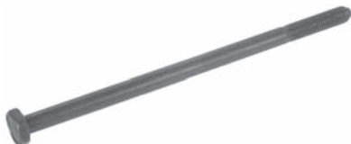
253426 Std pkg 10 Servicing V5 M7 x 133 mm, 27 mm thread Thru bolt
