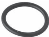
250628 Std pkg 10 Servicing 10P, 10PA, TV12C, -12EC, -14C 25 x 3 mm O-ring for oil seal (Neoprene) Same O-ring but HNBR: Cargo 250630
