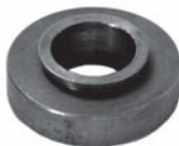
251441 Std pkg 10 Servicing A6, R4 O.D. 31.47 mm, I.D. 15.05 mm, Th. 10.35 mm Seal plate, steel
