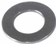
252319 Std pkg 10 Servicing V5 O.D. 27.68 mm, I.D. 15.75 mm, Th. 1.45 mm Thrust race
