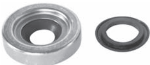
251514 Std pkg 5 Servicing DA6, HD6, HR6, HR6HE, HT6 O.D. 31.5 mm, I.D. 11.9 mm, Th. 8.5 mm Oil seal, double lip
