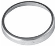
252745 Std pkg 10 Servicing R4 O.D. 32.65 mm, I.D. 28.48 mm, Th. 4.5 mm Felt wiper retainer
