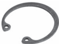
250613 Std pkg 10 Servicing DKV-14D For bore 28 mm, Th. 1.3 mm Retaining ring for oil seal (Beveled)
