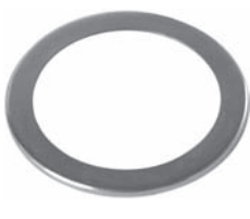
253358 Std pkg 5 Servicing 6CA17C O.D. 57.44 mm, I.D. 44.2 mm, Th. 2.33 mm Thrust race
