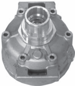
250852 Servicing V5 24.2 mm (front to retaining ring)
