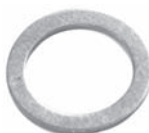
251861 Std pkg 10 Servicing DCW-17D O.D. 19.95 mm, I.D. 14.5 mm, Th. 0.8 mm Washer
