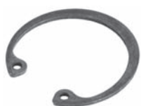
250613 Std pkg 10 Servicing CH, DKS-15BH, TM08-16 For bore 28 mm, Th. 1.3 mm Retaining ring for oil seal (Beveled)
