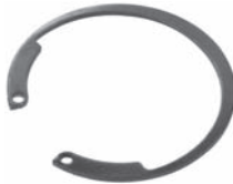
252120 Std pkg 10 Servicing SD7V16 For bore 55 mm, Th. 1.45 mm Retaining ring for pulley
