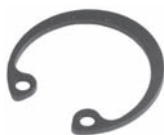
252530 Std pkg 10 Servicing 7SB16C For bore 21 mm, Th. 1 mm Retaining ring for oil seal
