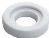
251442 Std pkg 10 Servicing A6, R4 O.D. 31.6 mm, I.D. 15.4 mm, Th. 7.5 mm Seal plate, ceramic
