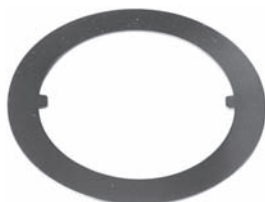
252030 Std pkg 10 Servicing SD508 O.D. 75 mm, I.D. 57.5 mm, Th. 0.8 mm Thrust race
