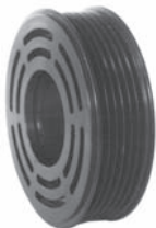
252392 Servicing SD7B10 O.D. 99 mm, bore 46 mm, W. 30.4 mm, 6 grooves
