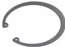
253263 Std pkg 10 Servicing SD508 For bore 63 mm, Th. 1.8 mm Retaining ring for pulley
