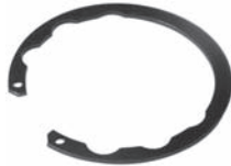
251752 Std pkg 10 Servicing SD7V16 For bore 55 mm, Th. 1.5 mm Retaining ring for pulley
