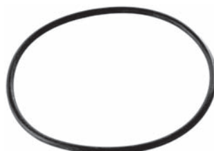
252676 Std pkg 10 91.67 x 3.53 mm O-ring for middle housing (Neoprene)
