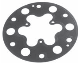
252445 Std pkg 10 Servicing SD6V12 O.D. 105.8 mm, Th. 0.4 mm Metal gasket - rear
