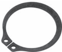
250623 Std pkg 10 Servicing FS6 For shaft 30 mm, Th. 1.2 mm Retaining ring for pulley / coil
