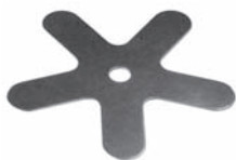
250610 Std pkg 5 Servicing SD505, -507, -508, -510, SD5H13, -14 Th. 0.6 mm Discharge valve reed
