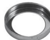
250733 Std pkg 10 Servicing BH O.D. 25.7 mm, I.D. 18.1 mm, Th. 4.3 mm Retaining ring for felt wiper
