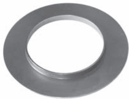
253299 Std pkg 10 Servicing 7SB16C O.D. 78.7 mm, I.D. 48.15 mm, Th. 1.2 mm Thrust race
