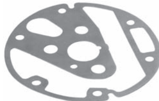
250766 Std pkg 10 Servicing DKS-17G O.D. 114 mm, Th. 0.6 mm Fiber gasket - front
