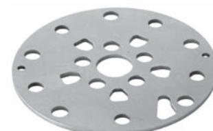
250019 Std pkg 10 Replacing 047151-0020 Servicing 10PA15C, -17C O.D. 105.5 mm, Th. 2.2 mm Valve plate - rear
