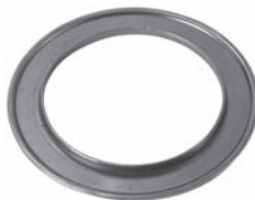
252371 Std pkg 10 Servicing DCW-17B O.D. 59.9 mm, I.D. 42.35 mm, Th. 3.34 mm Thrust race
