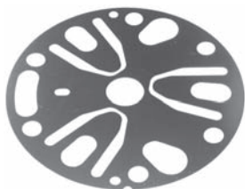
252431 Std pkg 10 Servicing DKS-15BH O.D. 109.8 mm, Th. 0.3 mm Suction valve reed
