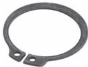
250041 Std pkg 10 Servicing MJ 110, MJS 170 For shaft 40 mm, Th. 1.5 mm Retaining ring for clutch coil
