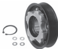
253410 Servicing 6SEU12C O.D. 110 mm, bore 51 mm, W. 35 mm, 6 grooves W/ hub
