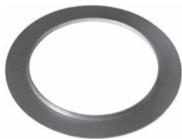
252029 Std pkg 10 Servicing SD508 O.D. 76 mm, I.D. 55.2 mm, Th. 0.8 mm Thrust race
