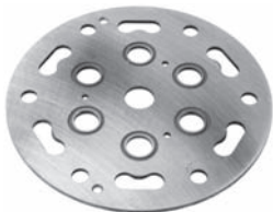
252236 Std pkg 10 Servicing SD6V12 O.D. 105 mm, Th. 2 mm Valve plate
