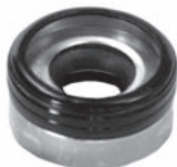
251176 Std pkg 5 Servicing DKV O.D. 30.25 mm, I.D. 13 mm, Th. 14.41 mm Oil seal w/ O-ring (HNBR)
