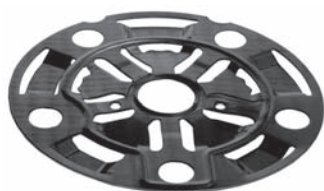
251393 Std pkg 10 Servicing FX15 1991 - 1992 O.D. 101 mm, Th. 0.9 mm Metal gasket - front / rear
