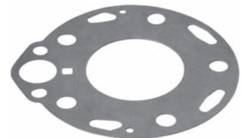
250742 Std pkg 10 Servicing DCW-17, -17B, -17D O.D. 120.5 mm, Th. 0.8 mm Fiber gasket - rear
