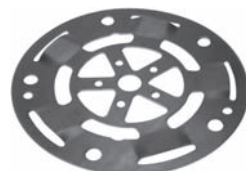
254102 Servicing 5SL12C-J O.D. 109.7 mm, Th. 0.8 mm Metal gasket
