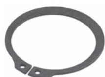
250092 Std pkg 10 Servicing BH, CH, DKS-17, DCW-17 For shaft 35 mm, Th. 1.3 mm Retaining ring for clutch coil (Beveled)
