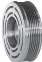
252498 Servicing SD508 O.D. 119 mm, bore 61.6 mm, W. 40 mm, 8 grooves
