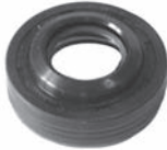
251566 Std pkg 5 Servicing V5, V7 O.D. 26.14 mm, I.D. 12 mm, Th. 10.3 mm Oil seal
