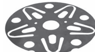
251084 Std pkg 10 Servicing FS10 O.D. 103 mm, Th. 0.3 mm Suction valve reed
