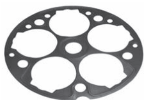
250600 Std pkg 5 Servicing SD505, -507, -508, -510, SD5H13, -14 O.D. 118 mm, Th. 0.7 mm Metal gasket - front
