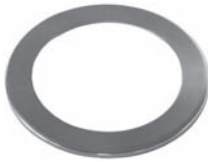
252329 Std pkg 10 Servicing SD6V12 O.D. 81.4 mm, I.D. 59.32 mm, Th. 3.3 mm Thrust race
