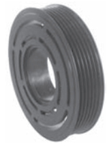
252305 Servicing DKS-15CH O.D. 119 mm, bore 50 mm, W. 27.7 mm, 6 grooves
