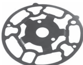
253063 Std pkg 10 Servicing 10S15C, -17C, -20C O.D. 109.7 mm, Th. 0.8 mm Metal gasket - rear
