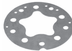
250595 Std pkg 5 Servicing SD507, -507, -508, -510, SD5H13, -14 O.D. 118 mm, Th. 1 mm Fiber gasket - rear
