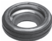
250874 Std pkg 5 Servicing V5 O.D. 26.3 mm, I.D. 12 mm, Th. 9.5 mm Oil seal
