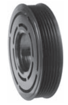
253325 Servicing DKS-17D O.D. 119 mm, bore 55 mm, W. 28.2 mm, 6 grooves
