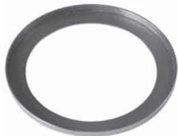
252317 Std pkg 10 Servicing V5 O.D. 76.8 mm, I.D. 59.2 mm, Th. 4.2 mm Thrust race
