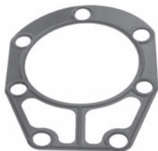
252518 Std pkg 10 Servicing RV2 Th. 0.3 mm Gasket for valve plate
