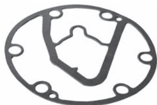
251224 Std pkg 10 Servicing 6P127, -148 O.D. 116 mm, Th. 0.85 mm Fiber gasket
