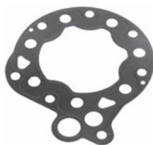
252915 Std pkg 10 Servicing SD7B10 O.D. 100.5 mm, Th. 0.37 mm Metal gasket - rear
