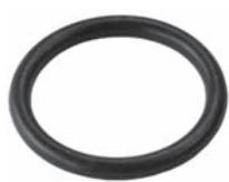
250753 Std pkg 10 Servicing DKS-13G, -17G 20.29 x 2.62 mm O-ring for suction port (Neoprene) Same O-ring but HNBR: Cargo 250477
