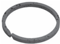
250342 Std pkg 10 Servicing A590, C171, 6E171, -171A O.D. 35.8 mm, Th. 2.77 mm Piston ring
