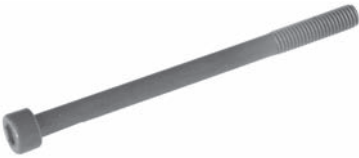
253267 Std pkg 10 Servicing 10PO8E M8 x 113 mm, 30 mm thread Thru bolt
