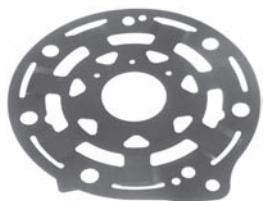
251919 Std pkg 10 Servicing 7SB16C O.D. 123.5 mm, Th. 0.8 mm Metal gasket - front
