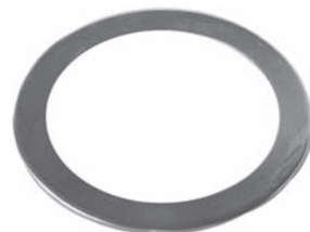
252368 Std pkg 10 Servicing 6CA17C O.D. 83.9 mm, I.D. 64.7 mm, Th. 2.2 mm Thrust race
