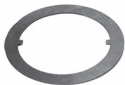
251810 Std pkg 10 Servicing SD7H15 O.D. 82.7 mm, I.D. 63.8 mm, Th. 1 mm Thrust race
