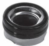
251166 Std pkg 5 O.D. 24.2 mm, I.D. 10 mm, Th. 11.9 mm Oil seal w/ O-ring (HNBR)
