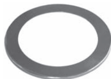
252328 Std pkg 10 Servicing SD7V16 O.D. 85.5 mm, I.D. 84.1/63.2 mm, Th. 3.3 mm Thrust race
