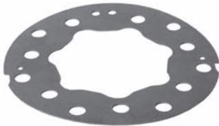
251501 Std pkg 10 Servicing SD7 O.D. 120 mm, Th. 0.85 mm Fiber gasket - rear
