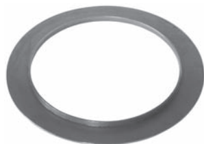
252307 Std pkg 10 Servicing SD7H15 O.D. 82.7 mm, I.D. 62 mm, Th. 0.8 mm Thrust race
