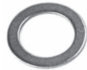
252690 Std pkg 10 Servicing FX80, -105V, -105VS O.D. 14.31 mm, I.D. 9.83 mm, Th. 0.71 mm Clutch shim
