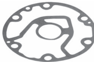
250783 Std pkg 10 Servicing DKS-16H O.D. 118 mm, Th. 1 mm Fiber gasket - front
