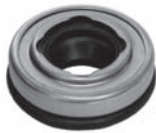
250325 Std pkg 5 Servicing V7 O.D. 30 mm, I.D. 10.7 mm, Th. 12.6 mm Oil seal w/ O-ring, lip type
