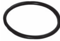
251257 Std pkg 10 Servicing TV10CB 23.52 x 1.78 mm O-ring for sensor, R134A only
