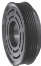
253322 Servicing SD7H15 O.D. 119 mm, bore 55 mm, W. 38 mm, 6 grooves
