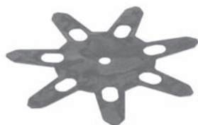
250089 Std pkg 10 Servicing SD708, -709, SD7V16 Th. 0.3 mm Suction valve reed
