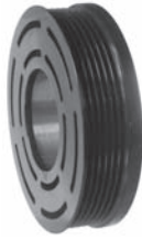
253326 Servicing 10P17C O.D. 123 mm, bore 62 mm, W. 32.5 mm, 6 grooves
