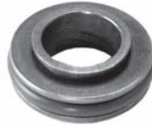
250650 Std pkg 5 Servicing FS6 O.D. 29.5 mm, I.D. 16.3 mm, Th. 10.7 mm Seal plate w/ extractor lip and O-ring (HNBR)
