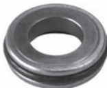
250194 Std pkg 5 Servicing SD708, -709 O.D. 27.5 mm, I.D. 15 mm, Th. 7.5 mm Seal plate, lip type w/ O-ring
