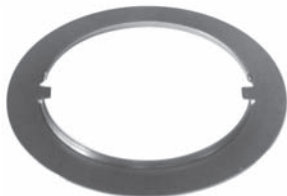
252158 Std pkg 10 Servicing SD7H15, SD709 O.D. 100 mm, I.D. 73.3 mm, Th. 0.8 mm Thrust race
