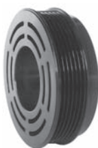
252383 Servicing V5 O.D. 119 mm, bore 62 mm, W. 41 mm 6 grooves
