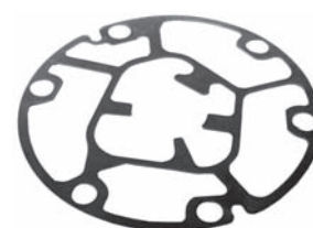
252828 OE Std pkg 10 Replacing 569310-2500 Servicing DKS-17CH O.D. 113.8 mm, Th. 0.5 mm Metal gasket - front
