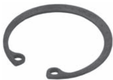
251280 Std pkg 10 Servicing Axial For bore 35 mm, Th. 1.5 mm Retaining ring
