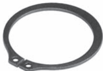
250581 Std pkg 10 Servicing DKV-14B, -C For shaft 35 mm, Th. 1.25 mm Retaining ring for pulley (Beveled)
