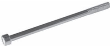
253305 Std pkg 10 Servicing 6P127B M8 x 132 mm, 28 mm thread Thru bolt
