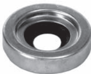
251478 Std pkg 5 Servicing DA6, HD6, HR6, HR6HE, R4, V5 O.D. 31.65 mm, I.D. 11 mm, Th. 7.5 mm Oil seal
