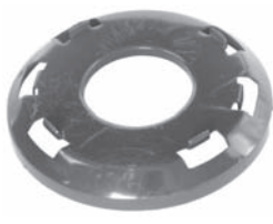
252405 Std pkg 10 Servicing 6CA17C O.D. 87.9 mm, I.D. 36.1 mm, Th. 16.1 mm Steel cover
