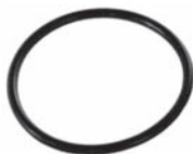
252603 Std pkg 10 28.3 x 1.78 mm O-ring for middle housing (Neoprene)
