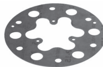
250227 Std pkg 5 Servicing SD6V12 O.D. 105.8 mm, Th. 0.8 mm Fiber gasket - rear
