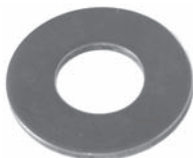
252353 Std pkg 10 Servicing V5 O.D. 34.3 mm, I.D. 16.1 mm, Th. 2.1 mm Thrust race
