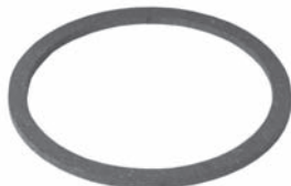
251616 Std pkg 5 Servicing 10P, 10PA O.D. 97 mm, I.D. 84.5 mm, Th. 3 mm Friction disc for pulley
