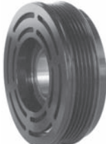
252495 Servicing SD508 O.D. 118.6 mm, bore 62.1 mm, W. 40 mm, 5 grooves
