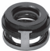
251440 Std pkg 10 Servicing A6, R4 O.D. 22.7 mm, I.D. 14.85 mm, Th. 17.1 mm Oil seal (HNBR)
