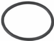
250604 Std pkg 10 Servicing SD5H13, -14, SD508, -510 29.5 x 2 mm O-ring for oil seal
