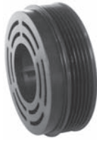
252395 Servicing V5 O.D. 125 mm, bore 62 mm, W. 41 mm 6 grooves
