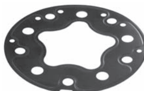
250147 Std pkg 5 Servicing SD505, -507, -507A2, -508, -510, SD5H13 O.D. 118.3 mm, Th. 0.7 mm Metal gasket - rear
