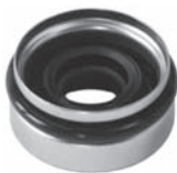
251027 Std pkg 5 Servicing NVR-140C, -140D O.D. 29.85 mm, I.D. 12 mm, Th. 12.45 mm Oil seal
