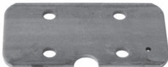
250171 Std pkg 5 Servicing FS6 L. 110 mm, W. 57 mm, Th. 3.3 mm Shipping plate
