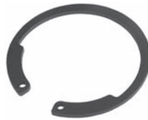
252026 Std pkg 10 Servicing SD508 For bore 62 mm, Th. 2 mm Retaining ring
