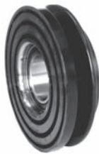
250861 Servicing V5 O.D. 131.5 mm, bore 62 mm, W. 40 mm, 1 groove Bearing: Cargo 250210
