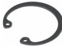
251683 Std pkg 10 Servicing SD508 For bore 28 mm, Th. 1.2 mm Retaining ring
