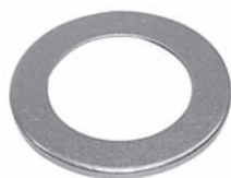
251854 Std pkg 10 Servicing SD7H15 O.D. 61.9 mm, I.D. 39.8 mm, Th. 0.9 mm Thrust race - rear
