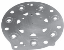
251955 Std pkg 10 Servicing 7SB16C O.D. 124.25 mm, Th. 2.23 mm Valve plate
