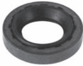
250548 Std pkg 10 A Servicing GM O.D. 30 mm, I.D. 15.6 mm, Th. 5.3 mm Manifold seal - thick type
