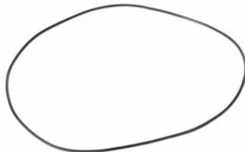
252634 Std pkg 10 133.07 x 1.78 mm O-ring for middle housing (Neoprene)
