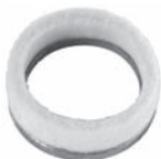
250108 Std pkg 10 Servicing SD708, -709, SD7H10 O.D. 30.6 mm, I.D. 23.2 mm Felt wiper
