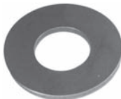
252728 Std pkg 10 Servicing V5 O.D. 35.35 mm, I.D. 16.1 mm, Th. 2.3 mm Thrust race
