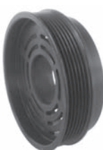
252549 Servicing FS10 O.D. 135 mm, bore 55 mm, W. 46 mm, 6 grooves
