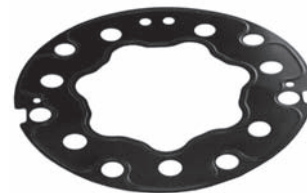
250202 Std pkg 5 Servicing SD708, -709 O.D. 120.5 mm, Th. 0.7 mm Metal gasket - rear
