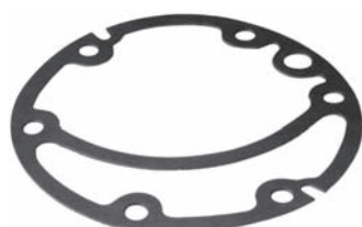
251009 Std pkg 10 Servicing DKS-13G, early models O.D. 110 mm, Th. 0.6 mm Fiber gasket - rear
