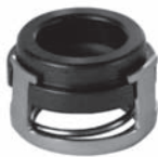
251157 Std pkg 5 Servicing N13A O.D. 22 mm, I.D. 13 mm, Th. 14.8 mm Oil seal w/ O-ring (HNBR)
