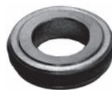
251213 Std pkg 10 Servicing FS6 O.D. 29.8 mm, I.D. 16.35 mm, Th. 7.98 mm Seal plate w/ O-ring (HNBR)
