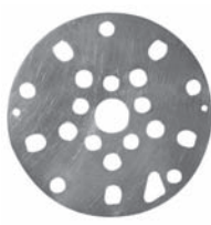
252153 Servicing 10PA20C O.D. 111.35 mm, Th. 2.25 mm Valve plate - rear
