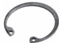
250680 Std pkg 10 Servicing 6CA17C, -17K, 10PO8E For bore 32 mm, Th. 1.2 mm Retaining ring for control valve (Beveled)
