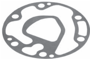
250722 Std pkg 10 Servicing DKS 15, BH Models O.D. 109.7 mm, Th. 0.6 mm Fiber gasket - rear
