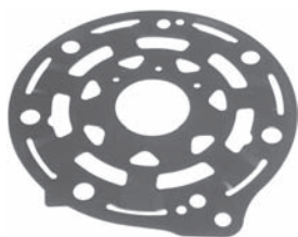
251918 Std pkg 10 Servicing 7SBU16C O.D. 123.5 mm, Th. 0.8 mm Metal gasket - front
