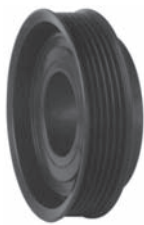
253116 Servicing SCS08 O.D. 115 mm, bore 52 mm, W. 39.7 mm, 6 grooves
