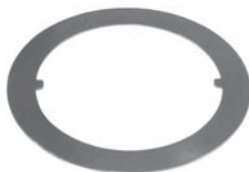
252032 Std pkg 10 Servicing SD507, -508, -510, -709, SD5H13, -14, SD7H15 O.D. 91.5 mm, I.D. 70.1 mm, Th. 0.8 mm Thrust race
