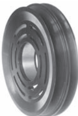
253317 Servicing SD709 O.D. 141 mm, bore 50.7 mm, W. 33.2 mm, 2 grooves
