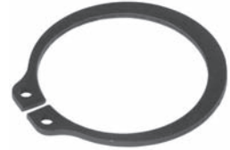
251682 Std pkg 10 Servicing SD508 For shaft 40 mm, Th. 1.8 mm Retaining ring
