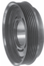
253310 Servicing DKV-11D O.D. 125 mm, bore 54.6 mm, W. 41 mm, 6 grooves
