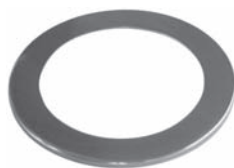
252308 Std pkg 10 Servicing SD7V12 O.D. 87.7 mm, I.D. 86.4/63.4 mm, Th. 3.3 mm Thrust race
