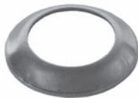
252174 Std pkg 10 A O.D. 19.4 mm, I.D. 12.6, Th. 3 mm (Beveled) Washer, copper
