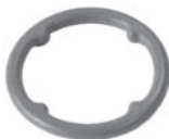
250429 Std pkg 10 Servicing 10PA Mercedes O.D. 24.5 mm, Th. 2.3 mm Manifold seal (HNBR)
