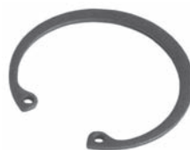
250151 Std pkg 10 Servicing 10P15C, -E, -F Mercedes, Toyota For bore 40 mm, Th. 1.6 mm Retaining ring for switch plug
