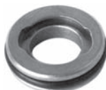
252698 Servicing SD505, -507, -575, TR70, -90, -105 O.D. 25.69 mm, I.D. 13.34 mm, Th. 6.71 mm Metal shaft seal seat w/ O-ring
