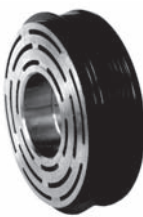
251378 Servicing V5 O.D. 142.5 mm, bore 62 mm, W. 39 mm, 6 grooves
