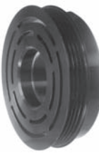
253318 Servicing DCW-17B O.D. 119 mm, bore 50 mm, W. 37 mm, 4 grooves
